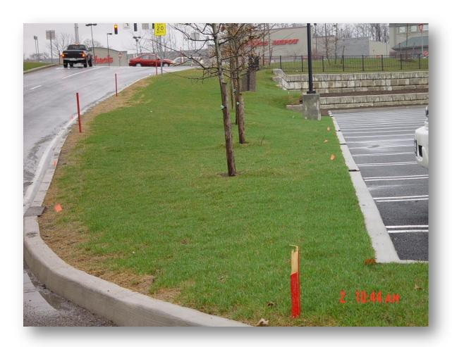
Figure 1 Damage from regular rock salt used on the roadways. The grass next to the parking area is not damaged due to Magic Salt was used on the parking area.
